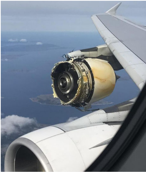
Fig. 1. The parts of engine that remained attached to the plane after the accident. Photo taken in-flight by passenger Enrique Guillen.
