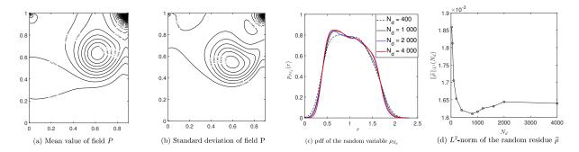
Figure 7: Reference unsteady stochastic flow at t = 30: (a) mean value  $\mathbf{x} \mapsto 1\ 000 \times m_P(\mathbf{x}, t)$ ; (b) standard deviation  $\mathbf{x} \mapsto 1\ 000 \times \sigma_P(\mathbf{x}, t)$ ; (c) pdf  $r \mapsto p_{PN_d}(r)$  of the random variable  $\rho_{N_d}$ ; (d)  $L^2$ -norm  $N_d \mapsto \|\widehat{\rho}\|_{L^2}(N_d)$  of the random residual  $\widehat{\rho}$ .
