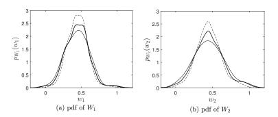
Figure 12: For  $N_d = 100$  and unsteady stochastic flow at t = 30, pdf  $w \mapsto p_{W_1}(w)$  (a) and pdf  $w \mapsto p_{W_2}(w)$  (b), estimated with the  $N_d = 100$  realizations (prior model) from the training dataset (solid line), with  $n_{MC} = 4\,000$  additional realizations (learning) estimated with the PLoM without constraint (dashed line) and under the constraints (thick solid line).
