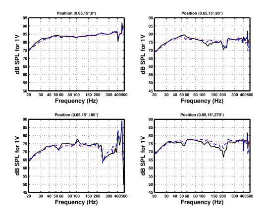
Fig. 10: Pressure levels (dB SPL) for 1 V at various positions (0.65,  $\theta$ ,  $\varphi$ ) on S for Sub1. Dotted lines: BEM processed from membrane velocities only, dashed lines: BEM processed from membrane and enclosure velocities, solid lines: FSM.
