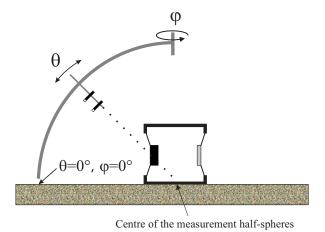
Fig. 2: Geometry of the measurement set-up.
