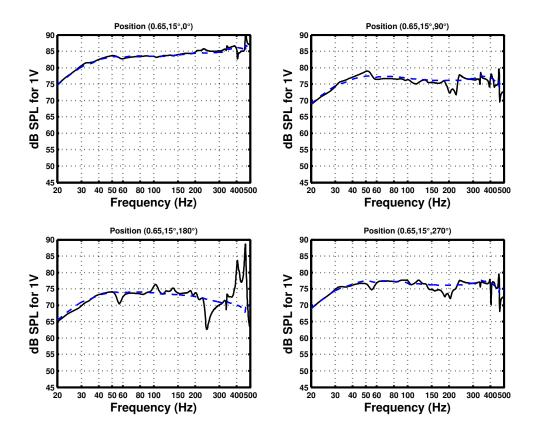
Fig. 8: Pressure levels (dB SPL) for 1 V at various positions (0.65,  $\theta$ ,  $\varphi$ ) on S for Sub1. Dashed lines: processed from membrane velocities only, solid lines: processed from enclosure and membrane velocities.
