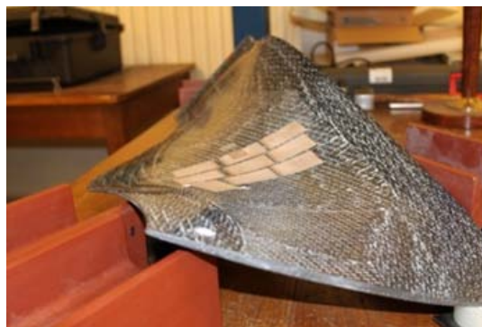
Figure 2: Patches mounted on the intrados
