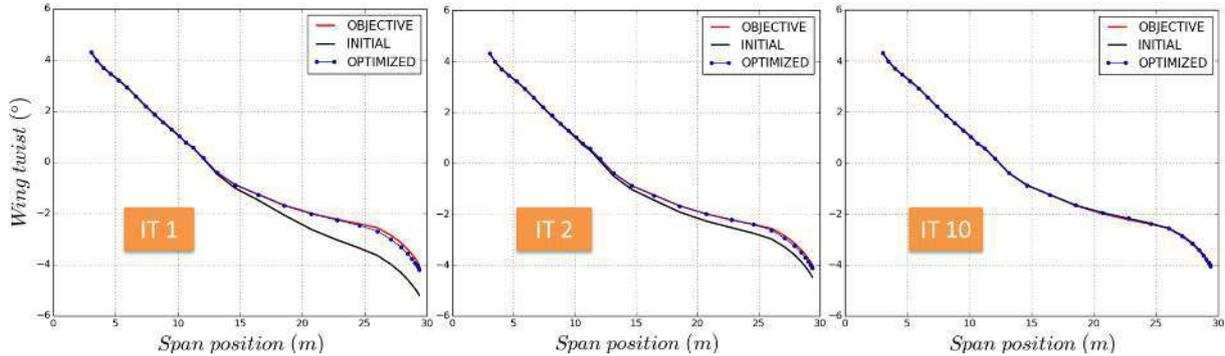
Figure 14: Initial (black), optimized (blue) and target (red) twist laws for three external iterations.
