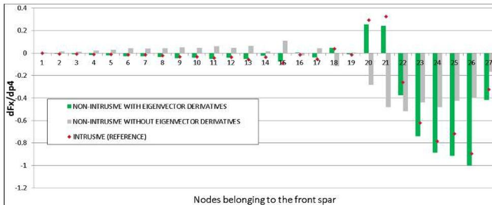
Figure 8: Gradients of horizontal force with respect to  $p_4$ , computed with the non-intrusive approach (green and grey bars). Reference tangent approach values (red markers) are provided.
