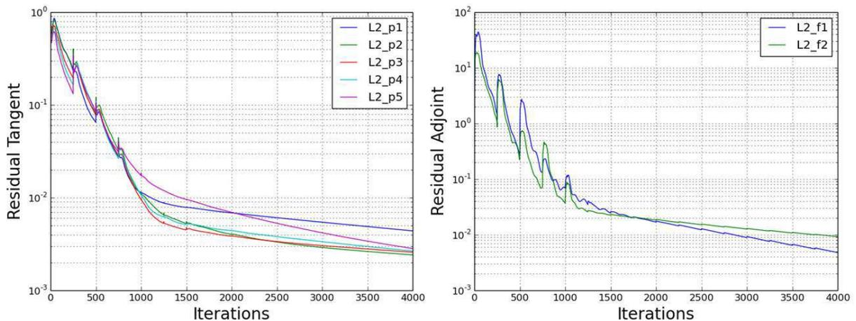
Figure 6: Convergence of linear gradient density residual for five parameters (left) and adjoint residual for two objective functions (right).
