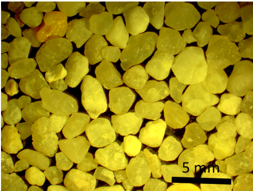
Figure 4. An image taken of the quartz sand under a microscope. The grains are much more angular and irregular than the spherical glass beads.
