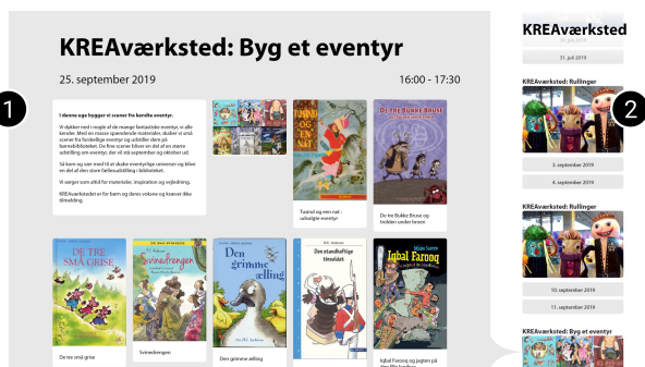
Figure 2. The visualization module retrieves content from the documentation module. ① On the left is the mosaic of content, ② on the right is the list of events.
