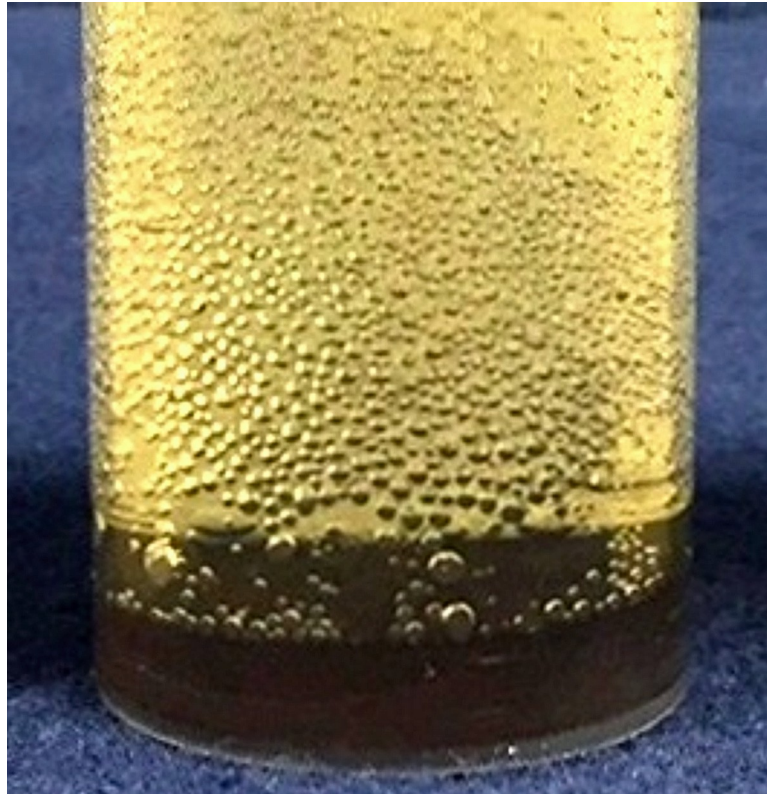
Fig 4. Example of gas generation. Bi 2 O 3 in NaOCl after 24 h, Light.
