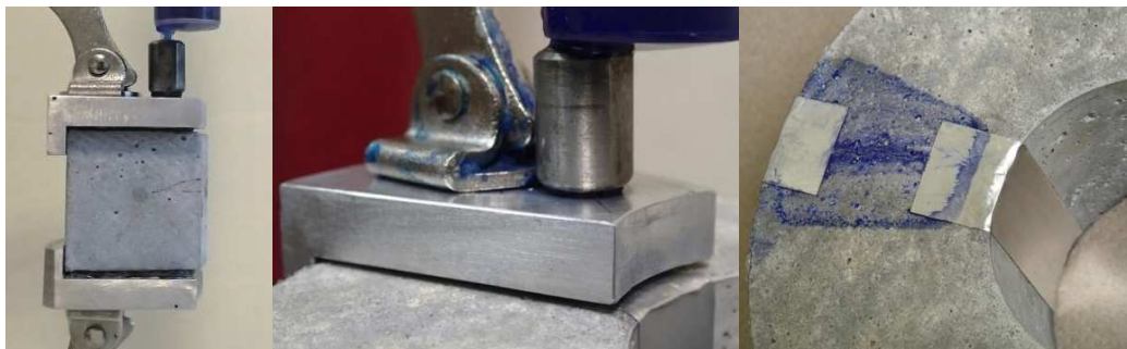
153 Fig. 1. From left to right – cross-sectional view of the injection device setup on a mortar sample; 154 upper side view; cracked mortar sample after injection of a colored solution
