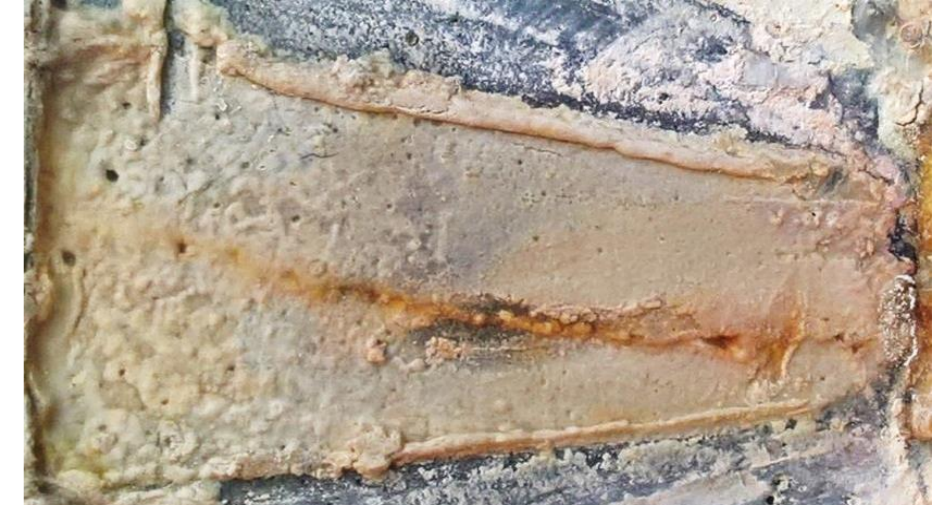
Composite (calcite – clay) clogging: Long-lasting crack repair
