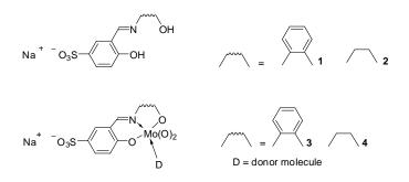
Scheme 1. Sulfonated tridentate Schiff base ligands NaH<sub>2</sub>L and the corresponding cisdioxidomolydenum(VI).
