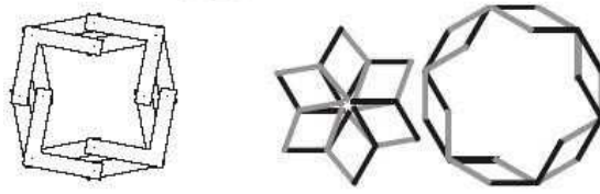
Fig. 3. Expanding "4-gon" and "6-gon" based on Hoberman design
