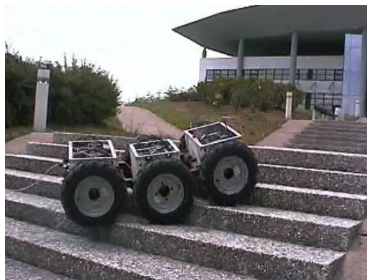
Fig. 1. The RobuRoc mobile robot climbing a stair
