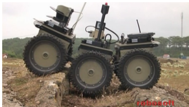
Fig. 1. RobuRoc6 negotiating an obstacle.
