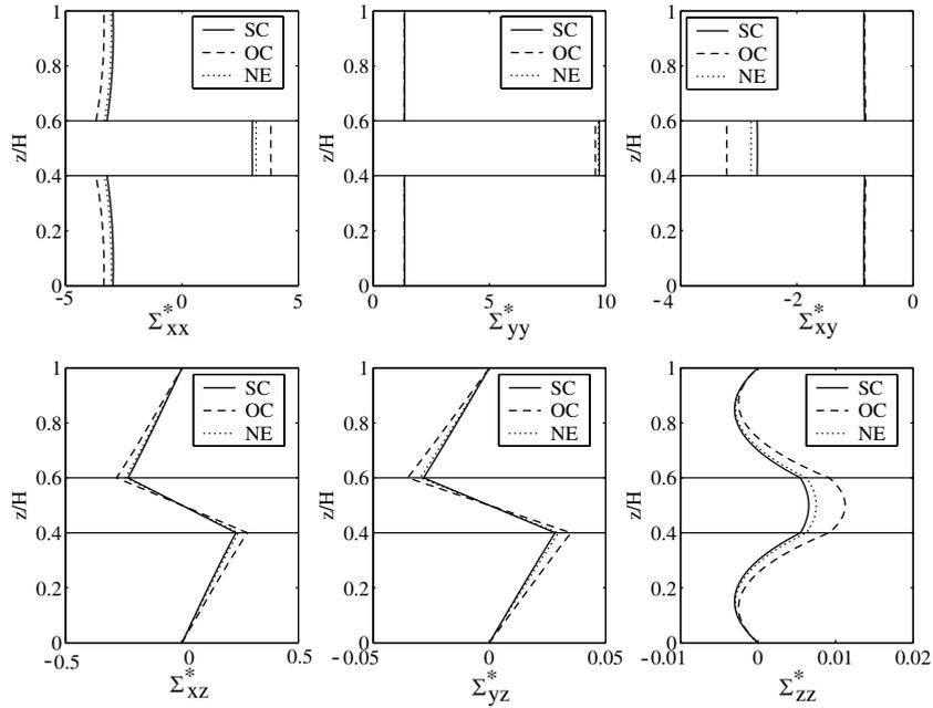
Fig. 11. Thickness distributions of the stresses for the thickness mode (1,1,2) of a SS shear-mode adaptive sandwich plate with different electric boundary conditions.
