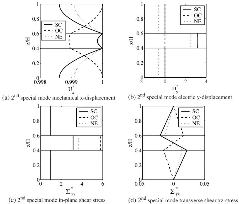
Fig. 7. Thickness distributions of *non-nil* mechanical and in-plane electric state variables for the special mode (0,1,2) of a SS shear-mode adaptive sandwich plate with different electric boundary conditions.
