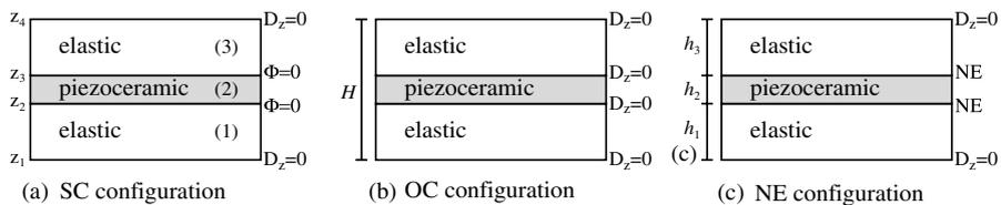
Fig. 3. A sandwich plate with SC/OC electroded or NE shear-mode piezoceramic core.
