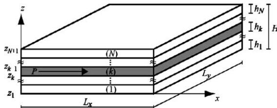
Fig. 1. Adaptive composite plate: polarization, geometry and notations.
