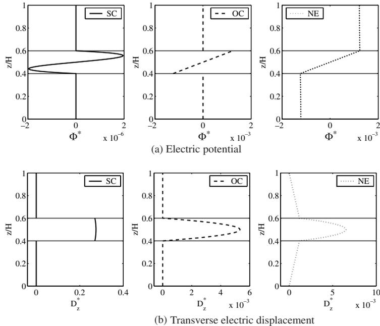
Fig. 5. Thickness distributions of electric potential and transverse electric displacement for the fundamental mode (1, 1, 1) of a SS shear-mode adaptive sandwich plate with different electric boundary conditions.
