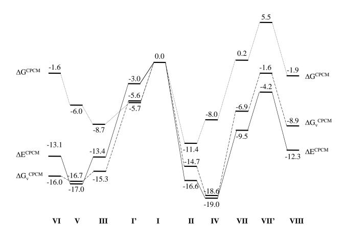
**Figure 2.** Energy diagram for the  $\Delta E^{CPCM}$  (plain lines),  $\Delta G_v^{CPCM}$  (dashed lines), and  $\Delta G^{CPCM}$  (dotted lines) approaches for the anionic model in dichloromethane at 25°C. All values are reported in kcal mol<sup>-1</sup> relative to **I**. Species **VII**' is a different conformer of **VII**, where one C<sub>2</sub>H<sub>4</sub> ligand has the C-C axis coplanar with the coordination plane [13].
