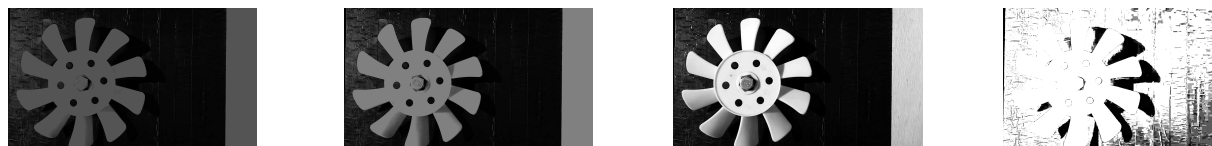
Figure 2: Gray-scale conversion using different formula. From left to right: Average, Lightness, Luminosity, Information
