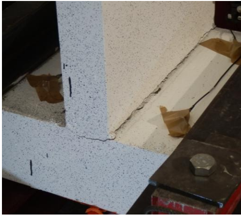
Figure 8 - Experimental and numerical deformation and crack pattern for specimen RC1-REF
