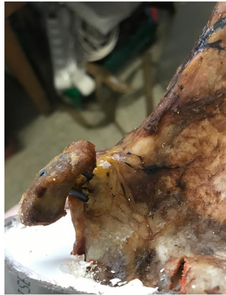
Fig. 4: One example of fixation failure : screws cut-out
