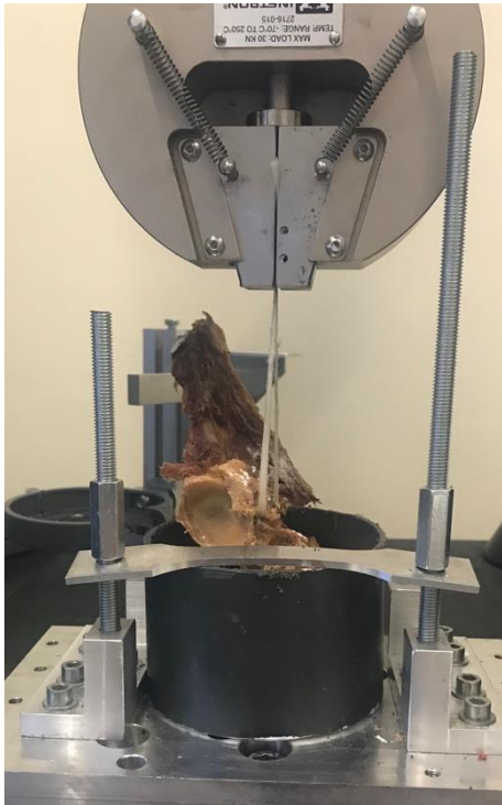
Fig.3: Positioning of the model before increasing tension test
