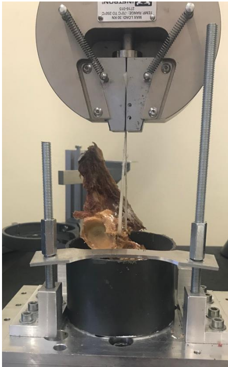
Fig.3: Positioning of the model before increasing tension test
