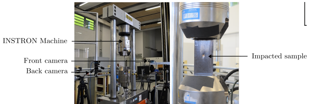
Figure 7: Fatigue tensile test on impacted sample
