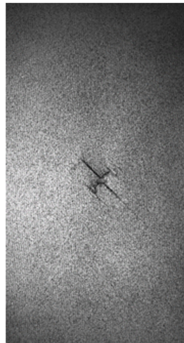
Figure 13: Fracture surfaces obtained after fatigue tensile test on impacted carbon woven laminate of configuration C45C45 with the lower impact energy and displacement level
