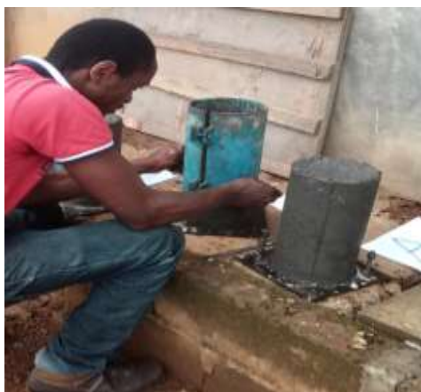
Figure 28 demolding of specimen
