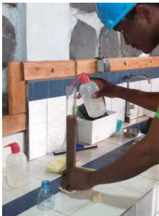
Figure 12 Rinsing the walls of the test piece
