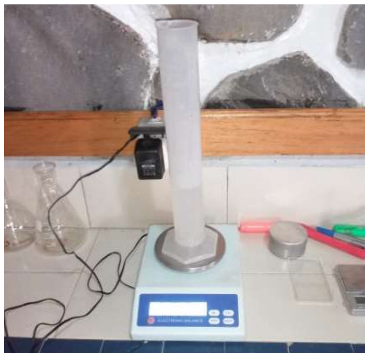
Figure 23 Weighing the specimen containing water
