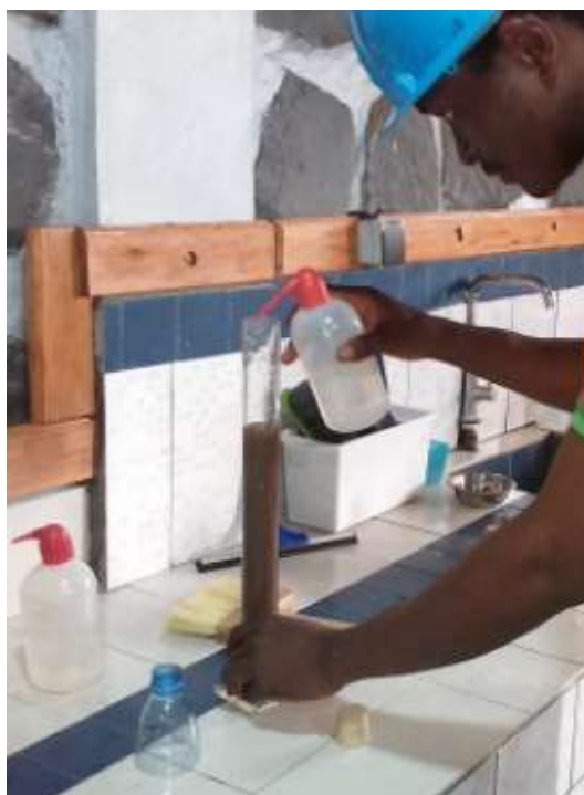
Figure 12 Rinsing the walls of the test piece
