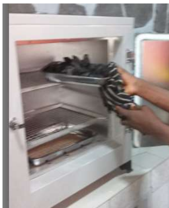
Figure 19 Drying of charcoal in an oven
