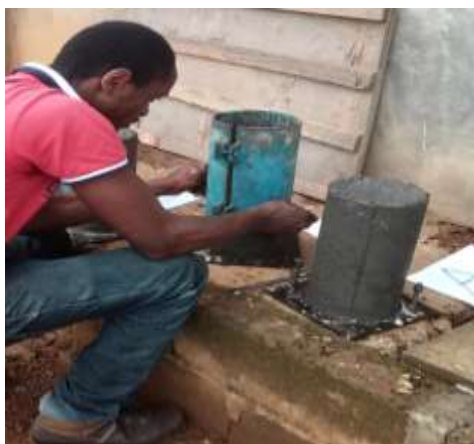
Figure 28 demolding of specimen
