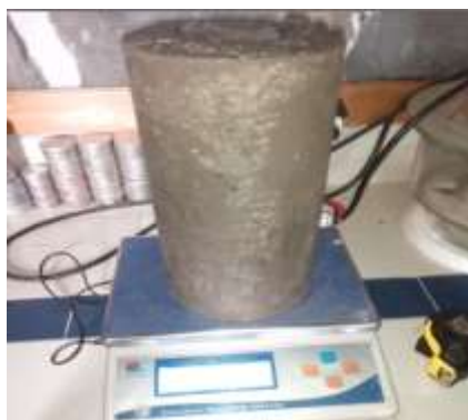
Figure 27 Measurement of the mass of the concrete
