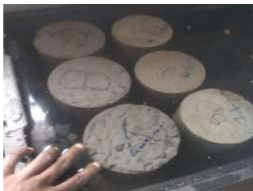
Figure 29 Immersion of concrete samples in water
