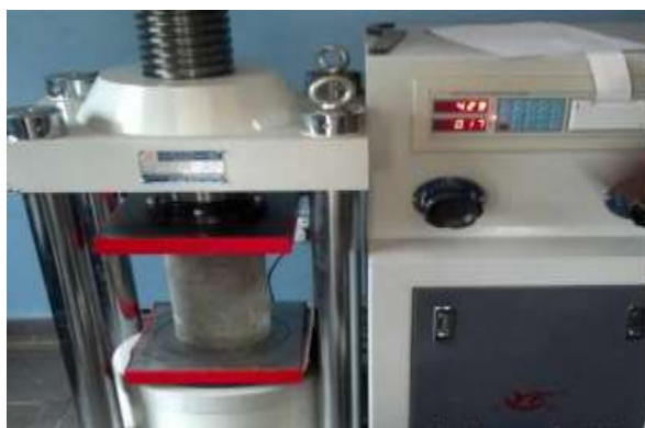
Figure 30 Compressive strength testing machine
