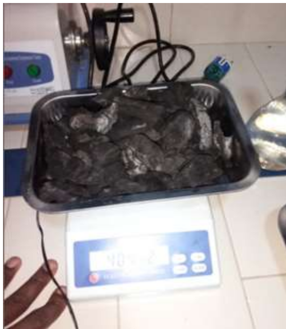
Figure 20 Weighing charcoal after drying
