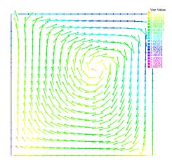
FIGURE 1. Numerical velocity (Driven cavity),  $\gamma = 10, \eta = 20$ .
