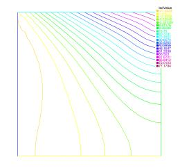
FIGURE 2. Numerical pressure (Driven cavity),  $\gamma = 10, \eta = 20$ .
