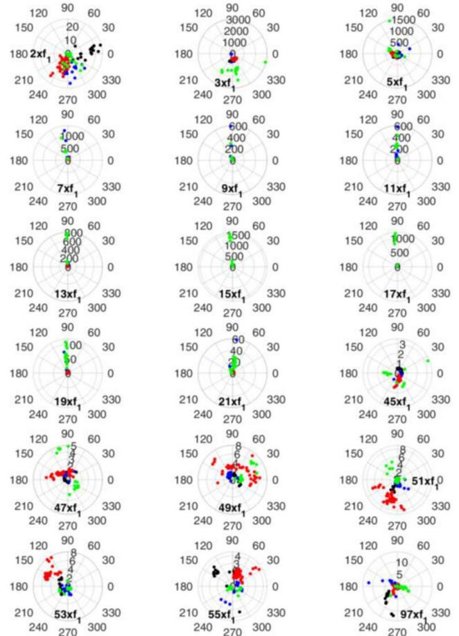
FIGURE 11  $P_h$ - $Q_h$  polar diagram for F 50 Hz harmonics: braking condition, four different time intervals (colour)
