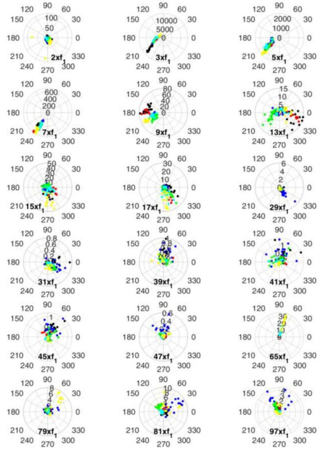
FIGURE 9  $P_h$ - $Q_h$  polar diagram for D 16.7 Hz harmonics: braking condition, six different time intervals (colour)
