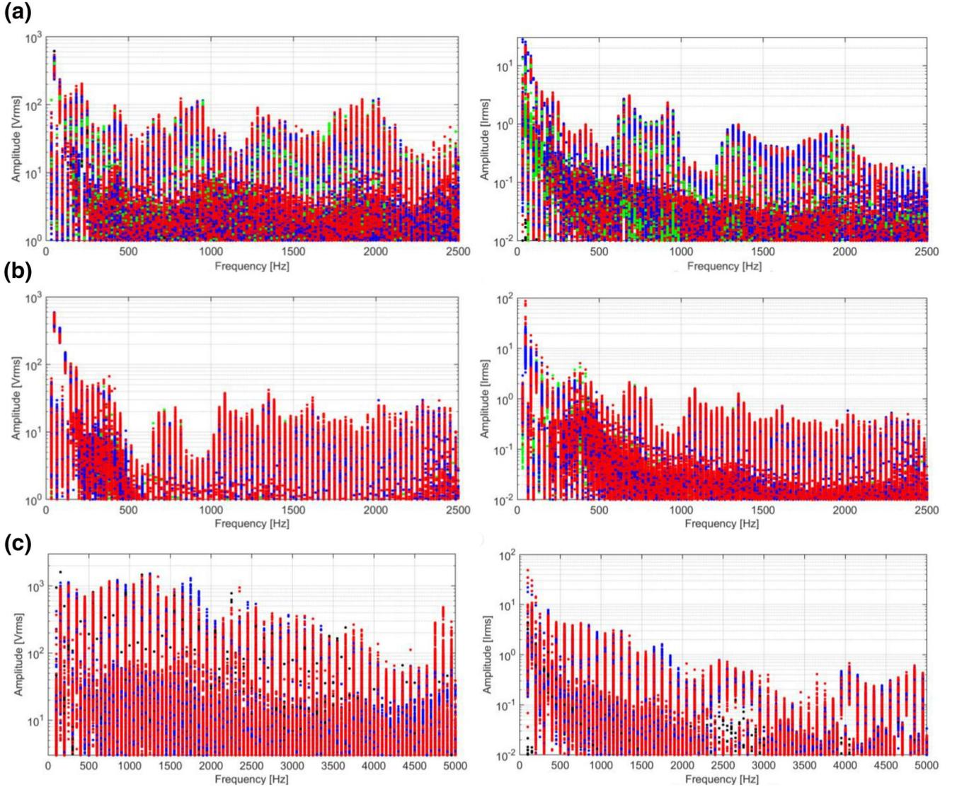
**FIGURE 2** Harmonic spectrum of  $V_p$  and  $I_p$  (traction in red, braking in blue, coasting in black and standstill in green): (a) 16.7 Hz system (Switzerland), (b) 16.7 Hz system (Germany), (c) 50 Hz system (France) [23].
