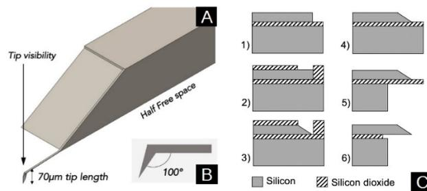
**Fig. 2.** A: Schematic view of the Lprobe cantilever and its holder. B: The angle between the tip and the cantilever let an optical path to see the tip end from the top. C: Process flow for Lprobe micro-fabrication. See main text for detailed steps.
