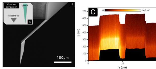
**Fig. 3.** A: On-scale comparison of tip aspect ratio between a standard tip (pyramidal shape) and the Lprobe tip. B: SEM image of the Lprobe cantilever and tip. C: Measured s-SNOM signal in the YZ plane. The black area is the sample topography. The detected signal is strong above the left branch with a maximum close to the gap, while almost no contrast compared to the substrate is observed on the right branch.
