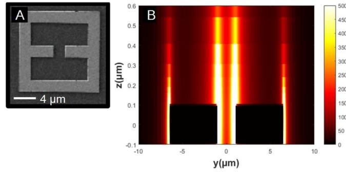
**Fig. 1.** A: SEM image of one of the fabricated SRRs. This work focuses on the field profile measurement along and above the axis of the central gap. B: Simulated and z-projected field intensity profile in the YZ plane, with Y being the axis of the gap and Z being the axis perpendicular to the substrate. The SRR is excited with a plane wave. As expected from the Curie's principle, the profile is symmetrical, and the intensity is the same on both sides of the gap.
