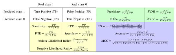
TABLE I: Some possible measures of the performance of a model. Measures in yellow quantify the *prediction* power of models, measures in green quantify the *correctness*, and those in blue quantify the *discrimination* power.
