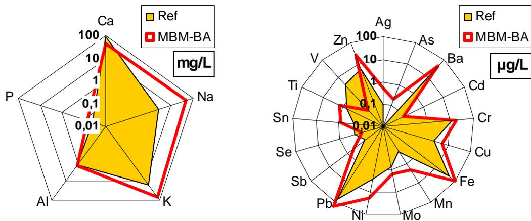
Figure 1. Quantity of elements leached from reference and MBM-BA mortars during leaching test on monolithic materials NF P31-211 (mg/L and  $\mu\text{g/L}$ ).
