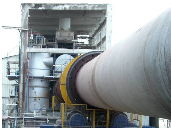
Figure 4 – Rotary kiln used for industrial scale tests
