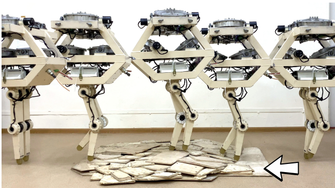
Fig. 4: The robot is able to walk "blindfolded" over small obstacles; no any kind of vision/remote sensing is used. Refer to Fig. 5 for a plot of the signals for this experiment.
