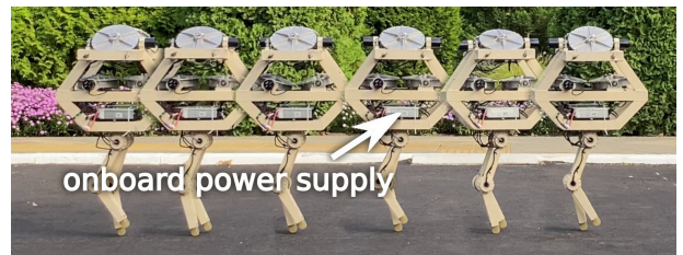
Fig. 8: gyrobot is meant to be autonomous, and is capable of walking outdoors. Even loaded with heavy batteries, no new control gains are needed!
