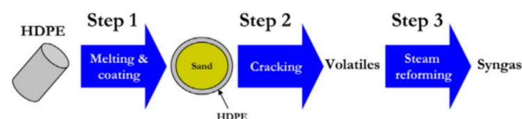
Figure 11. Steps in the gasification of plastics in a conical jet reactor. Reproduced from [67], Elsevier: 2013.
