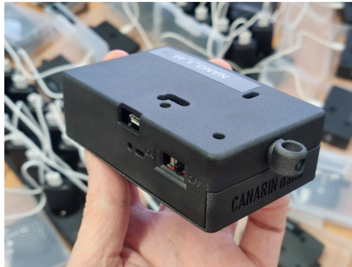
Figure 1. A Canarin Nano. The hook in the foreground is for carrying the device.
