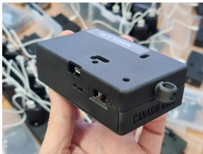
Figure 1. A Canarin Nano. The hook in the foreground is for carrying the device.
