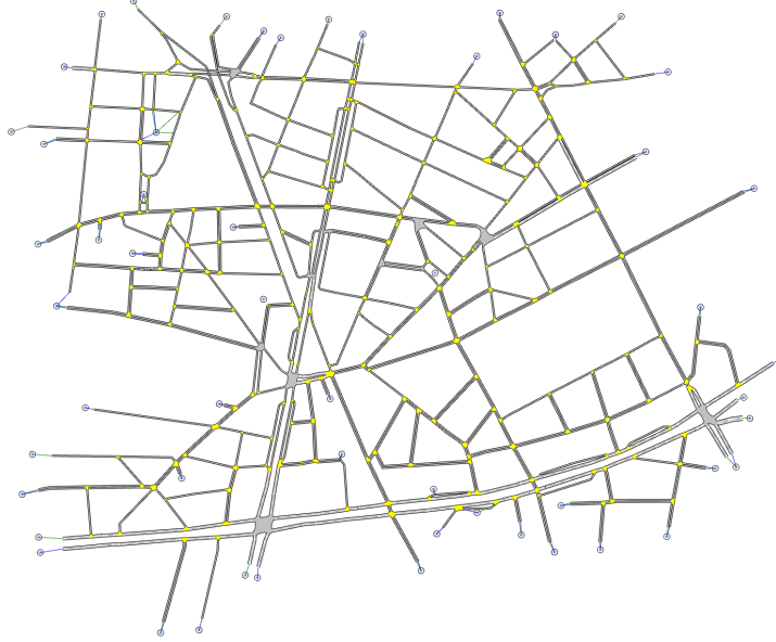
Figure 19: Recreated layout of the Grenoble network in Aimsun. For each road, parameters include the number of lanes, speed limit, length, and road interconnections.
