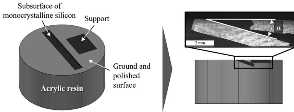
Fig. 4. Schematic diagram of embedded and bevel-polished specimen.
