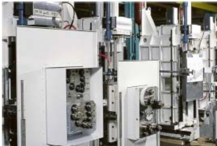
Figure 1. Multi-spindle equipment (PCI SCEMM, Groupe PSA)
