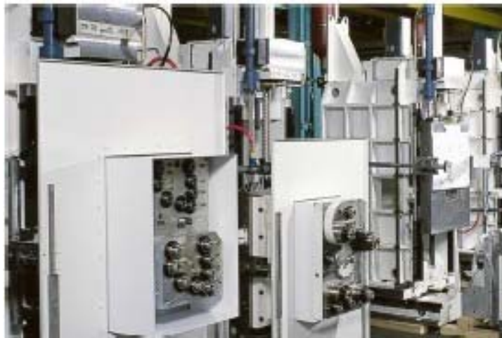
Figure 1. Multi-spindle equipment (PCI SCEMM, Groupe PSA)
