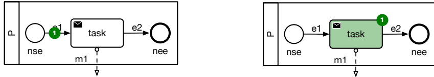
Figure 12: Starting behavior of a Send Task activity. Before (left) and after (right) application of the St rule.
