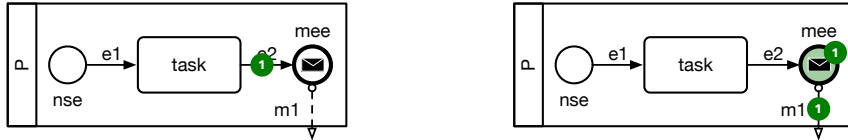
Figure 7: Starting behavior of a Message End Event. Before (left) and after (right) application of the St rule.
