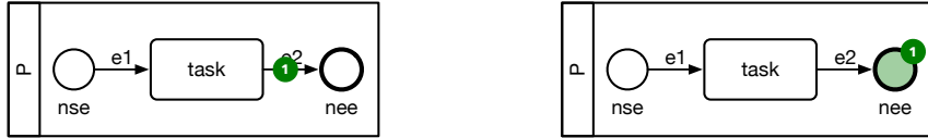
Figure 5: Starting behavior of None End Event. Before (left) and after (right) application of the St rule.
