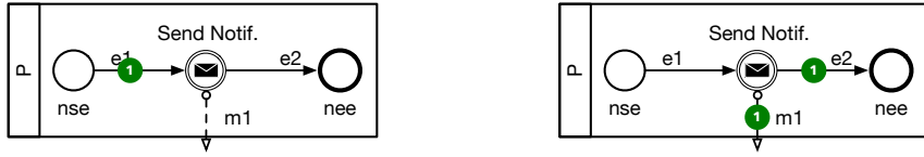
Figure 15: Starting behavior of a Throw Message Intermediate Event. Before (left) and after (right) application of the St rule.
