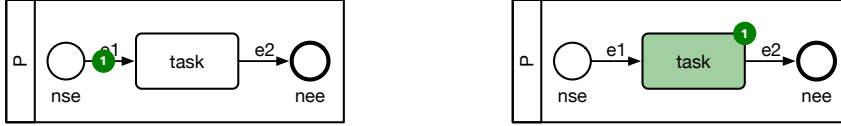
Figure 8: Starting behavior of an Abstract Task activity. Before (left) and after (right) application of the St rule.
