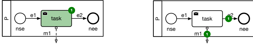
Figure 13: Completing behavior of a Send Task activity. Before (left) and after (right) application of the Ct rule.
