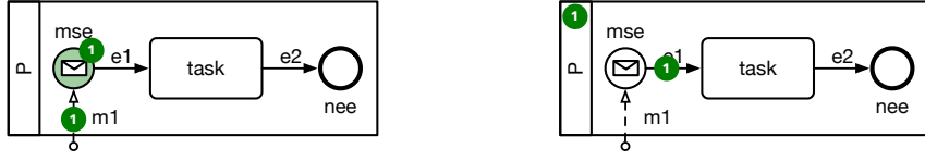
Figure 4: Completing behavior of a Message Start Event. Before (left) and after (right) application of the Ct rule.
