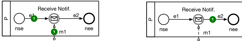
Figure 16: Starting behavior of a Catching Message Intermediate Event. Before (left) and after (right) application of the St rule.
