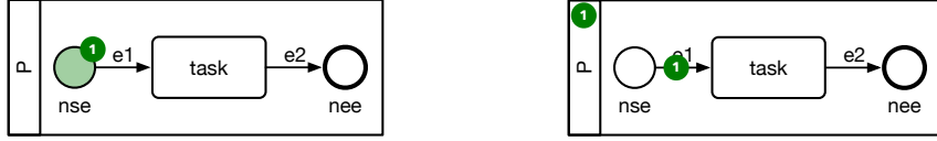
Figure 3: Completing behavior of a None Start Event. Before (left) and after (right) application of the Ct rule.
