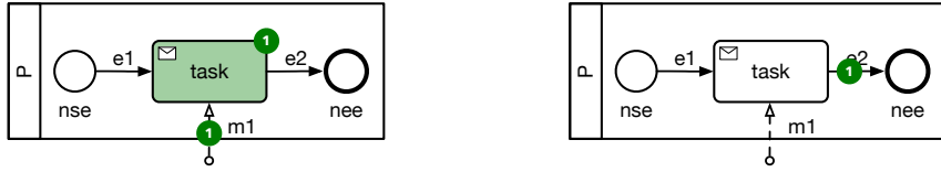
Figure 14: Completing behavior of a Receive Task activity. Before (left) and after (right) application of the Ct rule.
