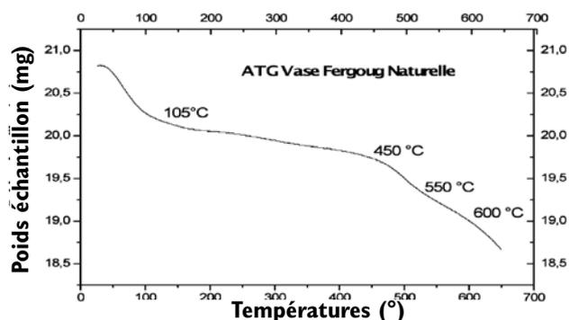
**Figure 2 : Courbe ATG de la vase de Feergoug crue**
