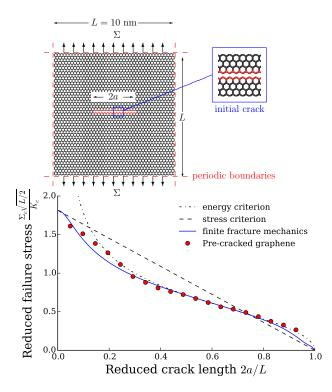
Figure 3: Remote stress at failure for 10 nm precracked periodic graphene systems in function of the crack length. Failure appears to be limited by strength at small crack lengths and by energy release at large crack lengths, which is reasonably captured by the initiation theory of FFM.
