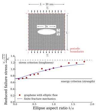
Figure 4: Remote stress at failure for 20 nm periodic graphene system with elliptic flaws in function of the aspect ratio of the flaw. The continuous transition from energy-driven failure at small aspect ratio to stress-driven failure at large aspect ratio is well captured by FFM.
