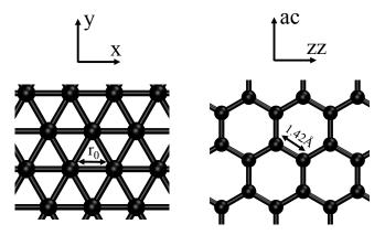
Figure 1: The two materials investigated : a toy model of triangular lattice (left), and graphene (right).
