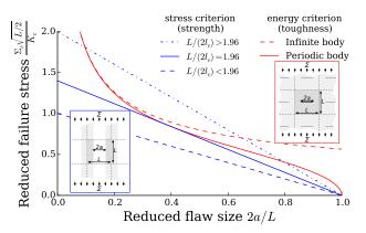
Figure 2: Relative position of of stress- and energydriven failure criteria for a periodic flawed material in function of the flaw and system size. The situation of interest for the study of size effects is when the relative positions of the criteria alternate which occurs if the system is large enough compared to the characteristic length  $l_c$ .
