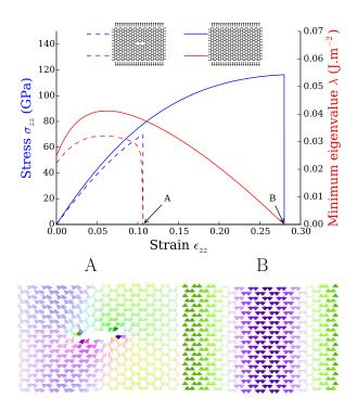
Figure 5: In the athermal limit, failure of graphene is an instability at the atomic scale (negative eigenvalue of the Hessian matrix), irrespective of the stress concentration. However, the mode of failure (eigenvector) strongly depends on the stress concentration.
