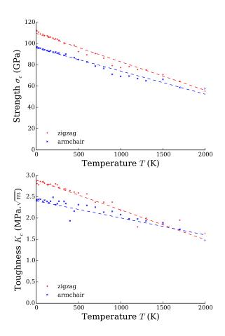
Figure 7: Strength and toughness of graphene as a function of temperature.
