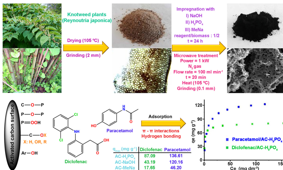
Fig. 7. Preparation of activated carbon by microwave heating using \text{H}_3\text{PO}_4 , \text{NaOH} , and sodium methanolate (MeNa) as the chemical agents, the activated carbon structure and its applicability for xenobiotics removal at optimal conditions (pH = 7, activated carbon dosage = 20 mg, time = 90 min, and temperature = 296 K). Reproduced with modification with permission from (Koutník et al., (2020)).
