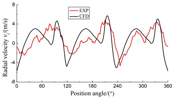
**Figure 12** The radial velocity for radius  $R=320\text{mm}$
