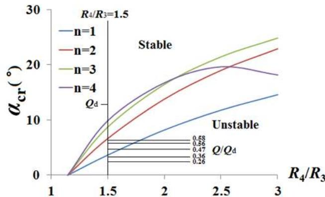
**Figure 2.** Critical flow angle versus diffuser ratio.
