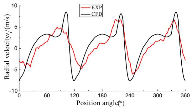
**Figure 13** The radial velocity for radius  $R=370\text{mm}$
