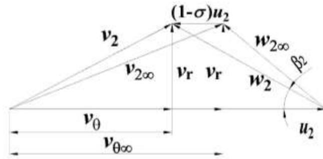
**Figure 3** Velocities' triangle at impeller's outlet
