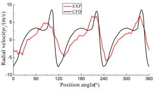
Figure 13 The radial velocity for radius R=370mm
