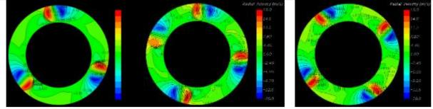
(a)  $Q/Q_d=0.26$  (b)  $Q/Q_d=0.31$  (c)  $Q/Q_d=0.61$ Figure 8 The radial velocity for different flow rates conditions
