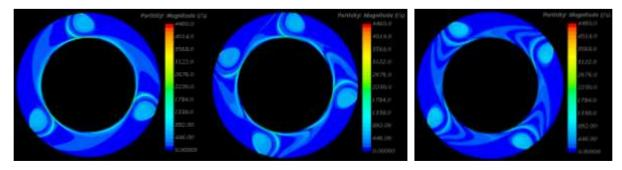
(a)  $Q/Q_d=0.26$  (b)  $Q/Q_d=0.31$  (c)  $Q/Q_d=0.61$ Figure 7 Vorticity magniture fields under different flow rates conditions
