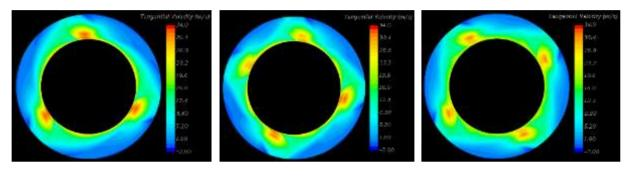
(a)  $Q/Q_d=0.26$  (b)  $Q/Q_d=0.31$  (c)  $Q/Q_d=0.61$ Figure 9 The tangential velocity for different flow rates conditions
