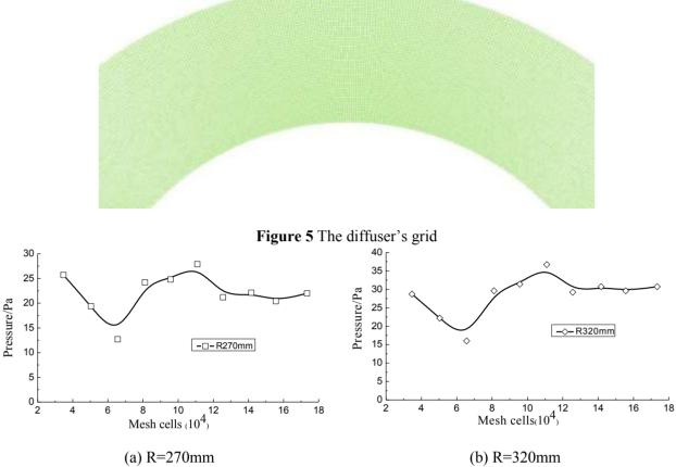
Figure 6 The amplitude of the peak spectrum for the dominant frequency at  $Q/Q_d=0.46$
