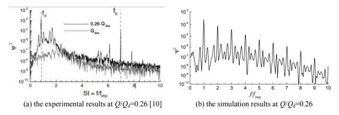
Figure 10 The spectral of pressure fluctuation
