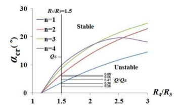
Figure 2. Critical flow angle versus diffuser ratio.
