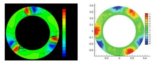
(a) calculation results (b) experimental results [11] **Figure 11** The radial velocity for the flow rate is  $Q/Q_d=0.26$
