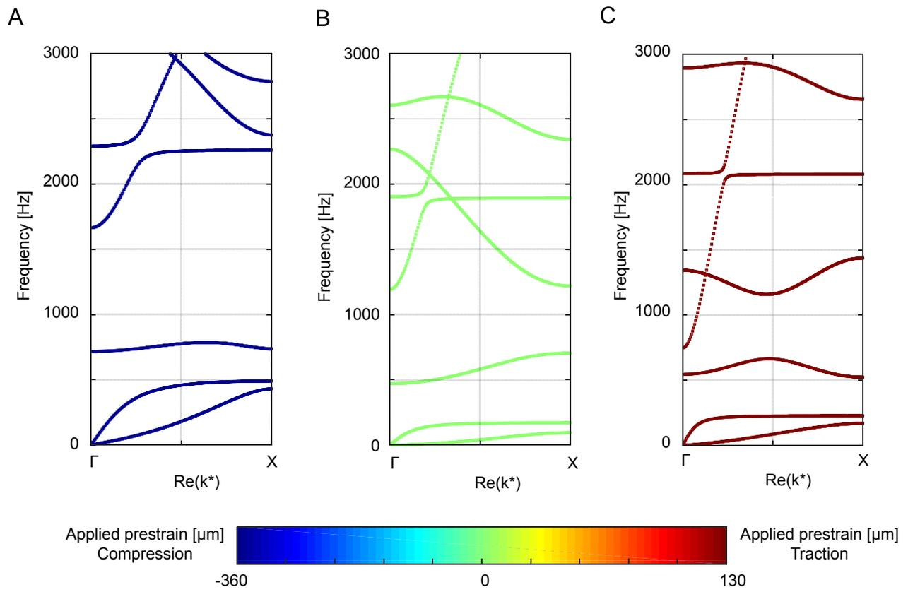
FIG. S1. **Plots of dispersion curves for single states of prestress.** Comparison of the dispersion curves plotted singularly for the (A)  $-360 \mu\text{m}$ , (B)  $0 \mu\text{m}$  and (C)  $+130 \mu\text{m}$  prestrain cases.
