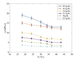
**Figure 5:** Viscosity of hemoglobin solutions as a function of temperature, measured by microrheology. Hemoglobin concentration ranges from 25.5 g/dL to 38.5 g/dL. Viscosity decreases with temperature and increases with concentration. For a given concentration range, viscosity values are spread over a wider range at low temperature than at high temperature.
