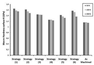
Fig. 9 Macro-hardness surface H (GPa) for different charge applications
