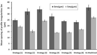
Fig. 8 Contribution of the six ball-burnishing strategies on the improvement of the mean spacing of profile irregularities Sm
