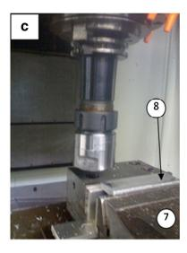
Strategy 6: Strategy ZIG/ZAG\_ SEUIL in two crossed passes, a first parallel ZIG/ZAG pass followed by a second perpendicular SEUIL pass to the milling direction (X-axis).
