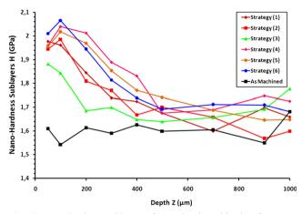
Fig. 10 Nano-hardness sublayers of treated and machined surfaces
