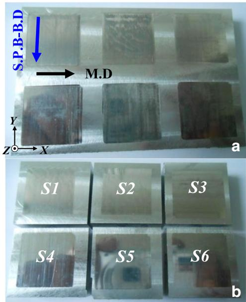
Fig. 4 Samples preparations: **a** application of the six ball-burnishing strategies, the second pass ball-burnishing direction (*S.P.B-B.D*), the milling direction (*M.D*); and **b** separation of the six ball-burnishing strategies for surface characterizations
