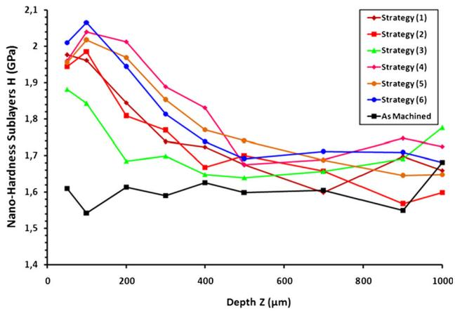
Fig. 10 Nano-hardness sublayers of treated and machined surfaces
