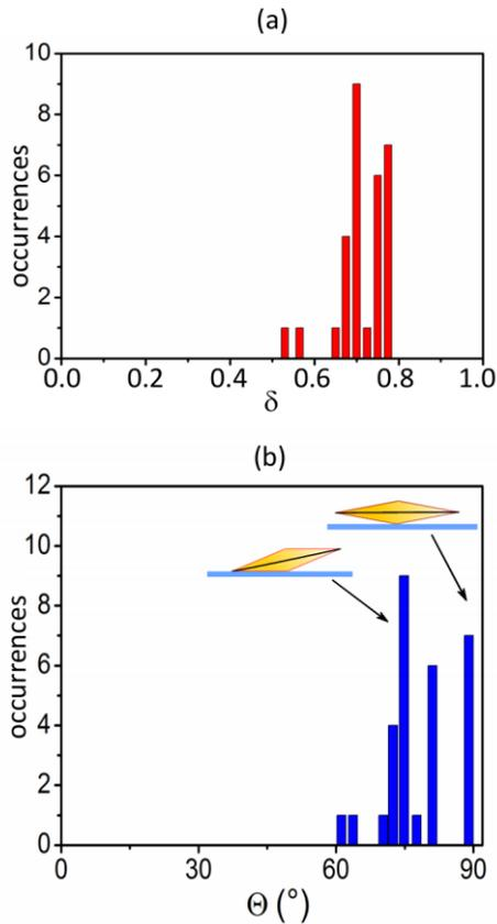
**Figure 3:** Histograms of (a) experimental values of  $\delta$ , and (b) deduced orientations  $\Theta$ , for 30 AuBP nanoparticles. Inset: Illustration of the AuBP orientations on the glass substrate.
