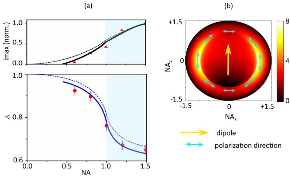
**Figure 4:** Evolution of the polarization measurement as a function of the objective numerical aperture: (a) degree of polarization  $\delta$  (below) and normalized maximum intensity  $I_{max}$  (above). Red dots are experimental measurements on the same single AuBP. The lines show two cases
