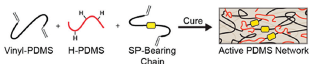
Fig. 22 Schematic representation of SP-containing PDMS network: synthesis route. 44 Fig. 22 is reprinted with permission from ref. 44, Copyright 2014 American Chemical Society.
