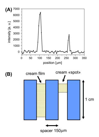
**Fig. 7.** (A) Step-by-step (5  $\mu$ m step) profile of a bilayer phantom two cream films separated by a 150  $\mu$ m glass slide. (B) Sketch not to scale of the bilayer phantom profiled in (A). The first film is 1 cm wide. Experimental details are given in Section 4.4. The total acquisition time is 45 minutes.
