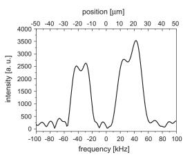
**Fig. 9.** Fourier transform of the echo obtained on a bilayer made of two thin films separated by a thin spacer of 20  $\mu$ m. The pulse length was of 4  $\mu$ s (see Section 4.4 for experimental details).
