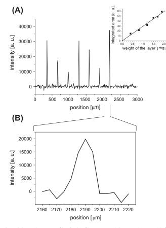
**Fig. 8.** (A) Step-by-step profile of a thin film cream multilayer. Each 1 cm wide film is separated by a glass slide of 150  $\mu$ m thickness. The step is 10  $\mu$ m (B) Step-by-step profile of the film of the 7th peak of the (A) multilayer. The step size is 5  $\mu$ m. Experimental details are given in Section 4.4.
