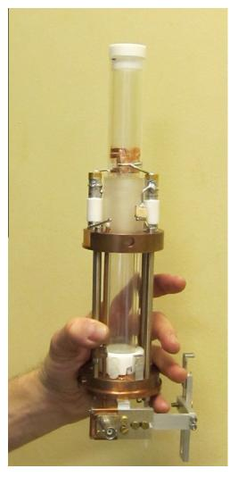
**Fig. 3.** Picture of our home-made STRAFI probe. The coil is made of copper strips sticked to a glass tube which crosses the whole probe. Thus, the sample positioned on top of a rod can move freely inside the glass tube whereas the probe is fixed against the superconducting magnet.
