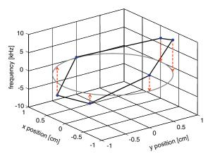
**Fig. 6.** Frequency shift (kHz) of an off-centered cream "spot" (1 mm diameter, 10  $\mu$ m thickness) versus the position of the sample holder (see Section 4.3). The position of the spot is 1 cm from the center. The tilt angle between the STRAFI plane and the sample plane is  $8 \times 10^{-4}$  rad.
