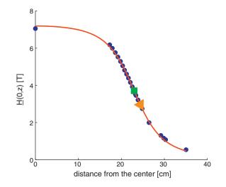
**Fig. 4.** Amplitude of the axial component of the magnetic induction of the superconducting magnet (points) used in this study and fit with a solenoid model (line) according to Eq. (16) (the fitting coefficients are I/2p = 3.7556 A/m, a = 0.0698 m et N.p/2 = 0.2298 m). The square represents the inflexion point and the left pointing triangle the theoretical position of the STRAFI plane of the solenoid model.
