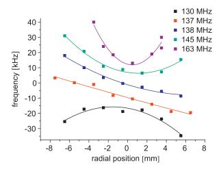
**Fig. 5.** Radial mapping of the magnetic field at various heights in the magnet. The figure is the plot of the frequency shift from a given base frequency (axial position) resulting from an off centered lateral motion. The acquisition protocol is described in Section 4.1.
