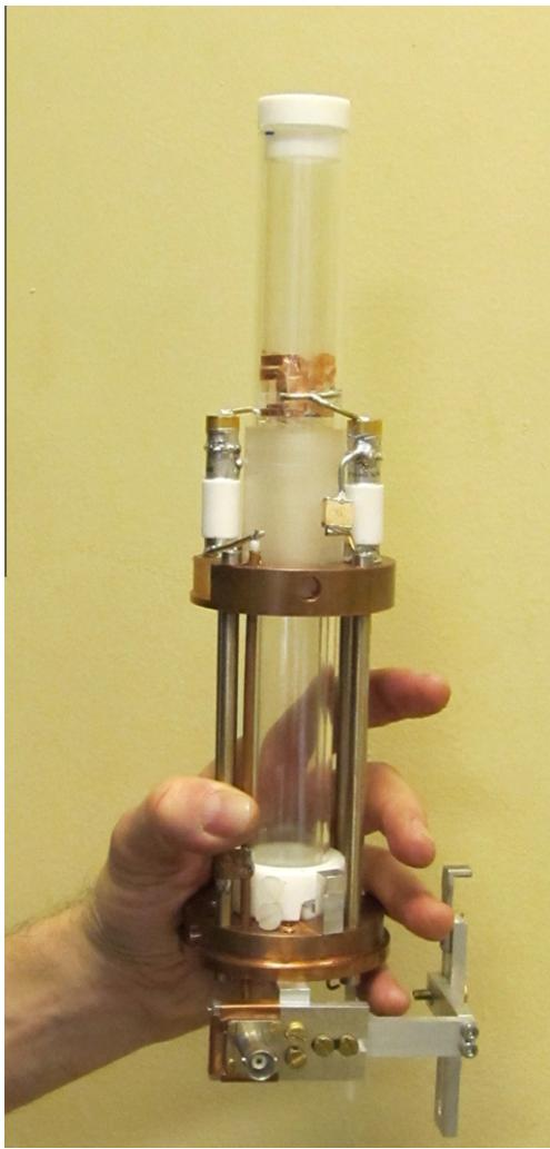
**Fig. 3.** Picture of our home-made STRAFI probe. The coil is made of copper strips stuck to a glass tube which crosses the whole probe. Thus, the sample positioned on top of a rod can move freely inside the glass tube whereas the probe is fixed against the superconducting magnet.
