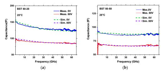
**Figure 6.** Comparison of measured and full-wave simulated IDC capacitance values versus frequency, for DC bias voltages of 0 V and 80 V, for the two BST compositions BST 80–20 (a) and BST 50–50 (b).
