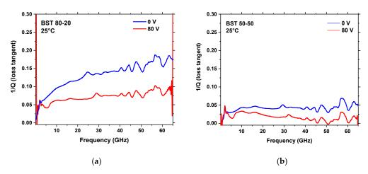
Figure 4. Overall losses of IDC devices integrating BST 80-20 (a) and BST 50-50 (b) for 0 V and 80 V applied bias.
