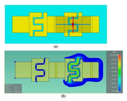
**Figure 5.** IDC topology used for the electromagnetic simulation, showing the position of the excitation discrete port (a) and amplitude of the electric field distribution in the device at 30 GHz (b).
