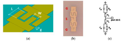
**Figure 1.** Topology of a typical metallic inter-digitated capacitor (IDC) structure on top of the ferroelectric (a), optical microscopy image of one of the fabricated device (b) and its equivalent electric scheme (c).
