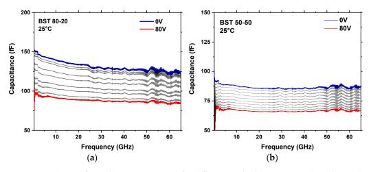
**Figure 2.** Frequency evolution of IDC device capacitances for different applied direct current (DC) bias voltages for the ferroelectric composition  $Ba_xSr_{1-x}TiO_3$  (BST) 80–20 (a) and BST 50–50 (b).
