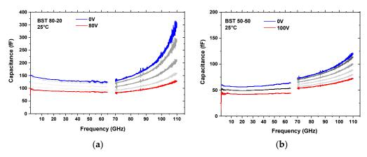
**Figure 7.** Capacitance values variation with applied bias for IDC devices integrating BST 80–20 (**a**) and BST 50–50 (**b**) thin films up to 110 GHz.
