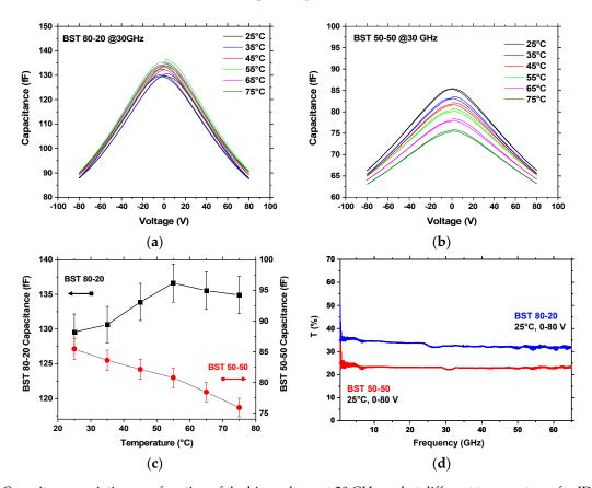
**Figure 3.** Capacitance variation as a function of the bias voltage at 30 GHz and at different temperatures for IDC devices integrating BST 80–20 (a) and BST 50–50 (b), evolution of the device capacitances at 30 GHz and 0 V bias with temperature (error bar amplitude at 2% of the measured value) (c), and room temperature frequency-dependent tunability T of both BST compositions at 133 kV/cm (d).
